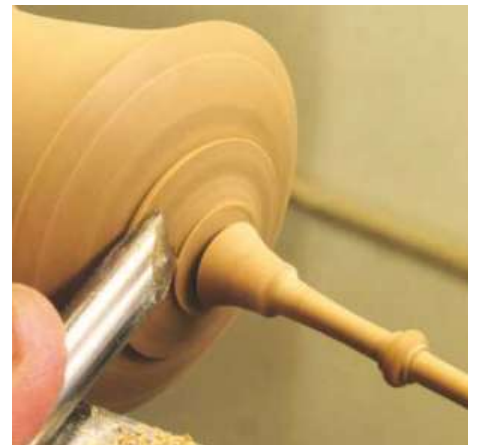
▲ Pic.24 After a couple of boxes Les is still not happy with the lid detail, cut with some difficulty with a skew, but he's hoping this can remain a secret between you and him
